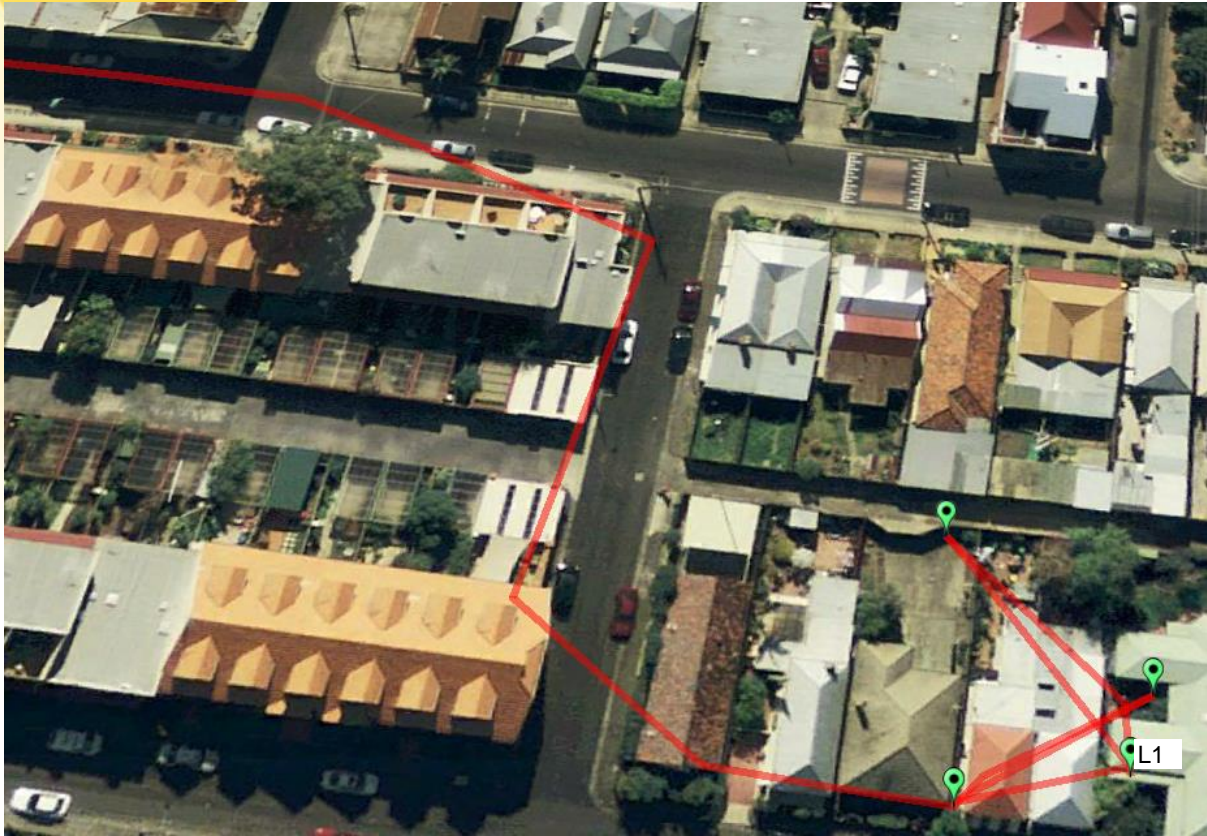
Figure 2 One of the TrackStick mini testing, with the device real position being Location 1 ('L1') inside a house at the bottom right corner
